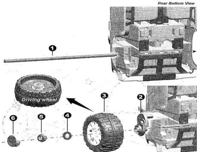
1. Unplug the wire connector from each gearbox in the battery area (one at a time). Remove gearbox from the battery area and install on the rear axle on the same side of the car. Make sure that the motor portion and wires slide into the hole in the body. Install wheel on the axle. Install washer and locking nut on the axle and tighten until snug. DO NOT overtighten. Install wheel center caps. REPEAT STEPS FOR OPPOSITE SIDE
