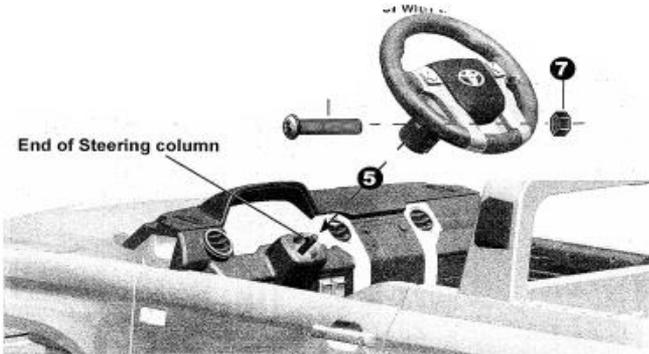
1. Remove the M5x35 machine screw and M5 nut from the steering wheel.
