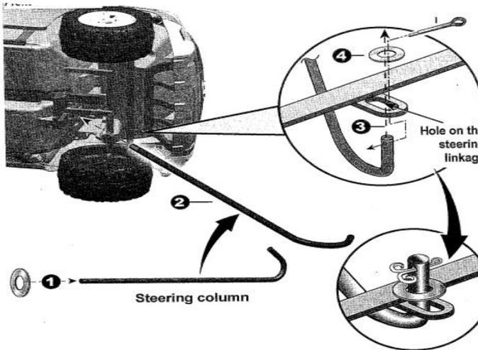
1. Slide a Washer on the steering column from the straight end. Insert the straight end of the steering column up through the hole on the front of the vehicle body from bottom side, and out through the hole on the dash. Insert the bent end of the steering column through the hole on the steering linkage.
